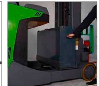
• The battery can be removed with the mast, and with side-way structure to facilitate the maintenance or replacement of the battery.
