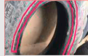
Bead Twisted And Deformed To Crack
