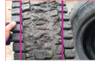
Pattern Block Cracking Or Dropping Off
